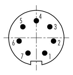
Contact arrangement (Plug-in side)
