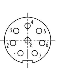
Contact arrangement (Plug-in side)
