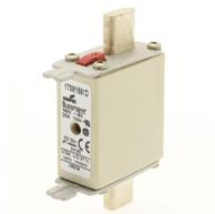
Fuse-link, high speed, 25 A, AC 690 V, DIN 000, gR, DIN, IEC, dual indicator, live gripping lugs
