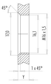
Installation direction: o-ring sits on chamfer.
