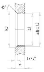
Installation direction: o-ring sits on chamfer.
