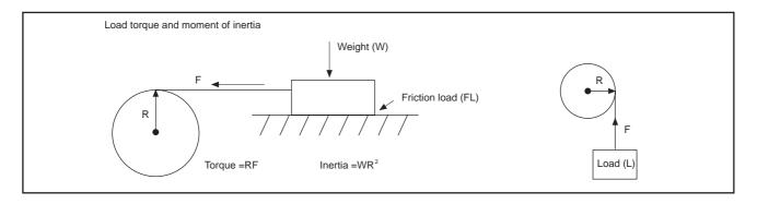
orque is the force (F) applied at a radius (R) to lift a Load (L) or overcome Friction (FL). Inertia is the tendency of a body weight (W) to preserve its state of rest or uniform motion in a straight line.
