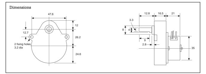
Gearbox parameters coupled with RS synchronous motor RS stock no. 440-385 at 50Hz
