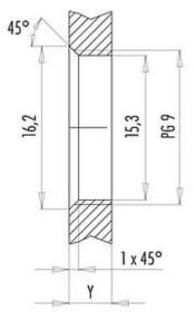
Installation direction: o-ring sits on chamfer.
