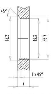
Installation direction: o-ring sits on chamfer.
