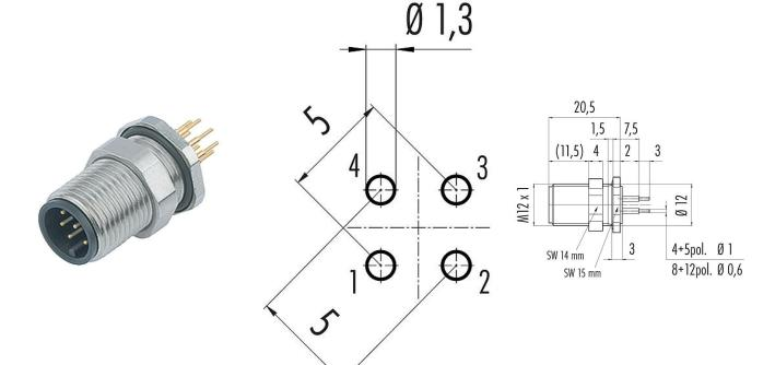
Contact arrangement (Plug-in side)
