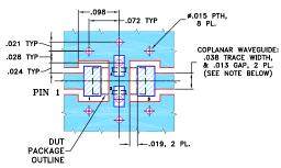
NOTES: 1. COPLANAR WAVEGUIDE PARAMETERS ARE SHOWN FOR ROGERS RO4350B WITH THICKNESS .020" ± .0015".
