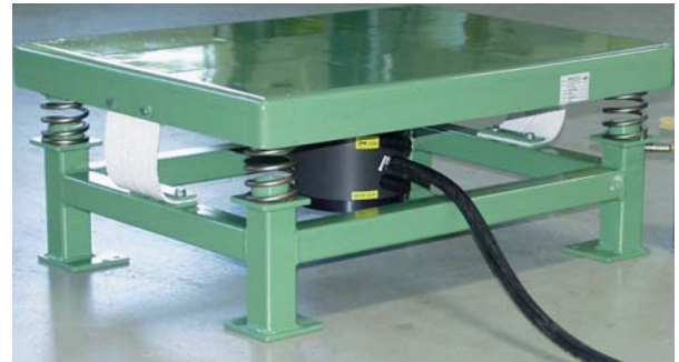
Compaction of powder in sacks
