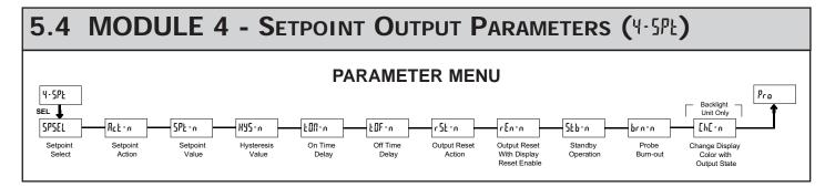
The Setpoint Output Parameters are only active when an optional output module is installed in the meter.
