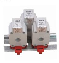
The compact current transformer is especially suitable for use in tight space conditions. With its primary 64 A it matches perfectly the 63 A with which domestic connections are usually fused. The secondary 1 A are connected to EFR3000. The inputs of the EFR3000 are preset for primary currents 60A, changing is simple. A clip for mounting on DIN-rail is included. The transformers can be clicked together for saving space. For EFR3000 three current transformers are required.
