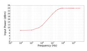
Figure 1. Max Input Operating Power vs Frequency
