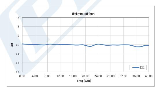
Click the following link (or enter part number in "SEARCH" on website) to obtain additional part information including price, inventory and certifications: 10 dB Fixed Attenuator, 2.92mm Male to 2.92mm Female Passivated Stainless Steel Body Rated to 1 Watt Up to 40 GHz PE7088-10
