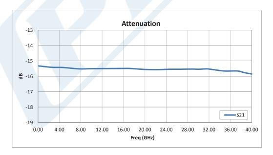
Click the following link (or enter part number in "SEARCH" on website) to obtain additional part information including price, inventory and certifications: 15 dB Fixed Attenuator, 2.92mm Male to 2.92mm Female Passivated Stainless Steel Body Rated to 1 Watt Up to 40 GHz PE7088-15
