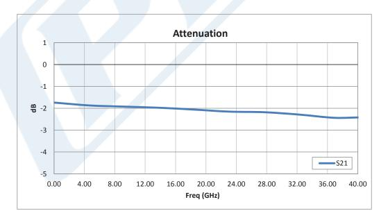
Click the following link (or enter part number in "SEARCH" on website) to obtain additional part information including price, inventory and certifications: 2 dB Fixed Attenuator, 2.92mm Male to 2.92mm Female Passivated Stainless Steel Body Rated to 1 Watt Up to 40 GHz PE7088-2
