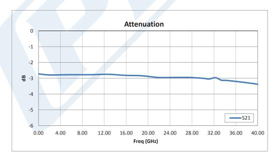
Click the following link (or enter part number in "SEARCH" on website) to obtain additional part information including price, inventory and certifications: 3 dB Fixed Attenuator, 2.92mm Male to 2.92mm Female Passivated Stainless Steel Body Rated to 1 Watt Up to 40 GHz PE7088-3
