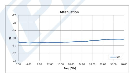
Click the following link (or enter part number in "SEARCH" on website) to obtain additional part information including price, inventory and certifications: 30 dB Fixed Attenuator, 2.92mm Male to 2.92mm Female Passivated Stainless Steel Body Rated to 1 Watt Up to 40 GHz PE7088-30
