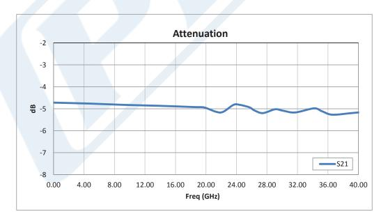
Click the following link (or enter part number in "SEARCH" on website) to obtain additional part information including price, inventory and certifications: 5 dB Fixed Attenuator, 2.92mm Male to 2.92mm Female Passivated Stainless Steel Body Rated to 1 Watt Up to 40 GHz PE7088-5
