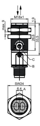
A Optical axis B Indicator diode
