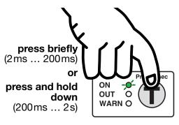
The **green** LED flashes **one time** quickly or for a longer period time after the button is pressed
