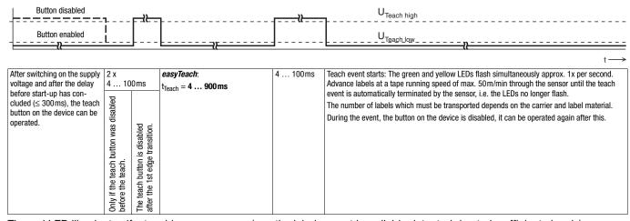
The red LED illuminates if a teaching error occurs (e.g. the label cannot be reliably detected due to insufficient signals). Regardless of the state, the green LED illuminates upon conclusion of the teach event; the yellow LED indicates the current switching state.
