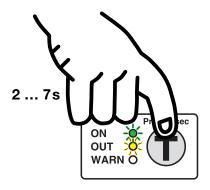
The **green** and the **yellow** LEDs flash **synchronously** approx. **1**x per sec.
