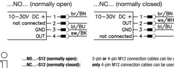
3-pin or 4-pin M12 connection cables can be used. only 4-pin M12 connection cables can be used.
