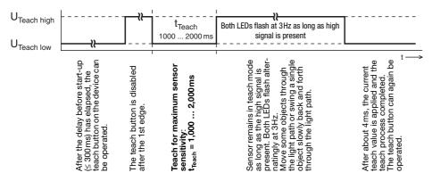
In the event of a teach error (e.g. no teach object or a teach object which is too small or too transparent is moved through the light path), the two LEDs flash at the same rate. Check the system, repeat the teach process, if necessary use a larger or less transparent teach object.
