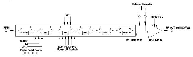
Figure 3. The DVGA1-242+ Serial interface consists of 6 control bits that select the desired attenuation state, as shown in Table 2 Truth Table.
