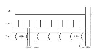
Figure 4. Serial Interface Timing Diagram
