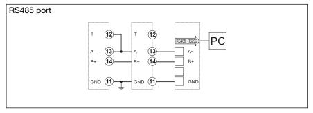
**RS485 NOTE:** additional devices provided with RS485 are connected in parallel. The termination of the serial output is carried out only on the last instrument of the network, by means of a jumper between (A-) and (T).
