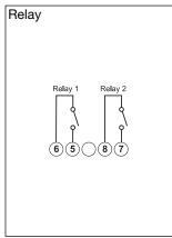
The load resistances (RC) must be designed so that the close contact current is lower than 100mA; the VDC voltage must be lower than or equal to 30VDC.
