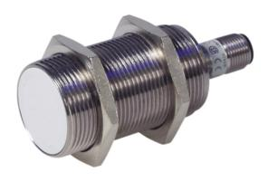
IA Series Inductive Proximity Sensors, nickel-plated brass M30 long housing, 18 to 30 V DC power supply, analogue current output 20-4 mA, 10mm sensing range, IP67 rating, 2m pre-wired cable
