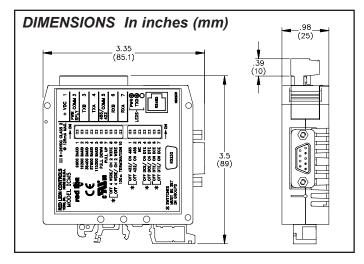
The unit is equipped with a universal mounting foot for attachment to standard DIN style mounting rails, including top hat profile rail according to EN 50 022 - 35x7.5 and 35x15, and G profile rail according to EN 50 035 - G32.
