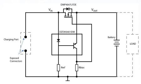
$V_{\text{IN}} > V_{\text{OUT}}$  minimizes forward losses.
