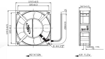
Frame:Aluminum Alloy Impeller:Plastic(UL:94V-0) Motor Structure:Shaded Pole Induction Motor. Rotational direction CCW looking at rotor. Lead wire:UL1430AWG22 Wire Type:-AT Terminal/ -AW Wires OPERATING TEMP\*:-10°C~70°C \*:-10°C~60°C for fans with sleeve/ball combination bearings.
