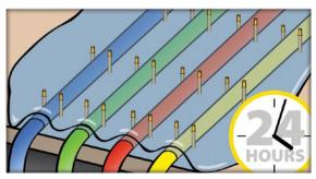
2. Multiple pours are needed to get proper thickness, and the molded cable takes 24-48 hours to fully cure.
