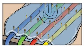
1. Wires are stretched between pins in a mold, and then liquid silicone plus additives are poured over the wires.
