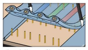
3. The cured cable is cut out of the mold, leaving sharp edges and multiple holes.
