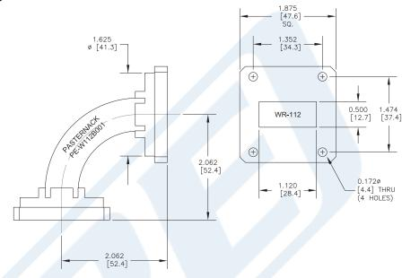
WR-112 Waveguide E-Bend with UG-51/U Flange Operating from 7.05 GHz to 10 GHz from Pasternack Enterprises has same day shipment for domestic and International orders. Our RF, microwave and millimeter wave products maintain a 99% availability and are part of the broadest selection in the industry.
