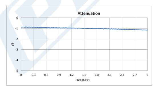
Click the following link (or enter part number in "SEARCH" on website) to obtain additional part information including price, inventory and certifications: 1 dB Fixed Attenuator, N Male to N Female Brass Nickel Body Rated to 1 Watt Up to 3 GHz PE7002-1
