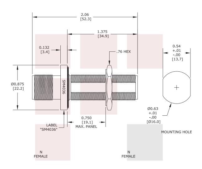
$\begin{array}{cc} \underline{\text{STANDARD TOLERANCES}} \\ .X & \pm 0.2 \\ .XX & \pm 0.1 \end{array}$
