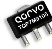
3-pin SOT-89 Package
