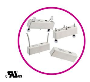
The DA(UL) series is a UL\* approved very high isolation voltages (up to 10kV) are achieved through the use of high vacuum reed switches with either rhodium or tungsten contacts and make these relays suitable for high reliability applications, such as cardiac defibrillators, test equipment and high voltage power supplies.
