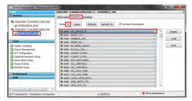
Figure 3-30. Verifying DS90UB95x Register
