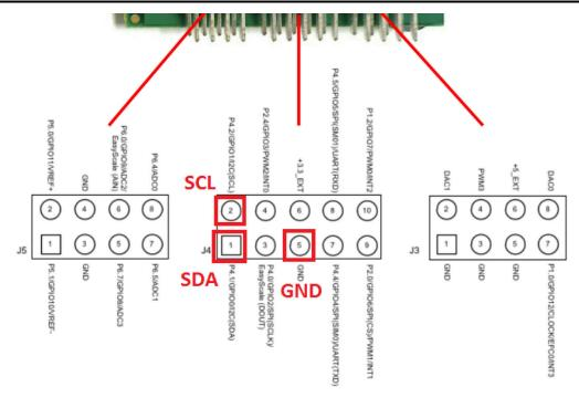
Figure 3-2. I2C Pinout of USB2ANY Connector
