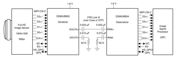
Figure 2-1. Typical Application Block Diagram Using DS90UB953-Q1 and DS90UB954-Q1 (or variant)
