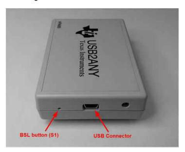
Figure 3-29. USB2ANY With Enclosure
