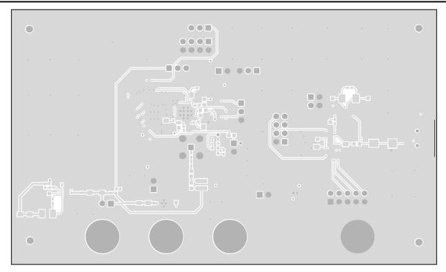
Figure 6-9. Bottom Layer PCB Layout
