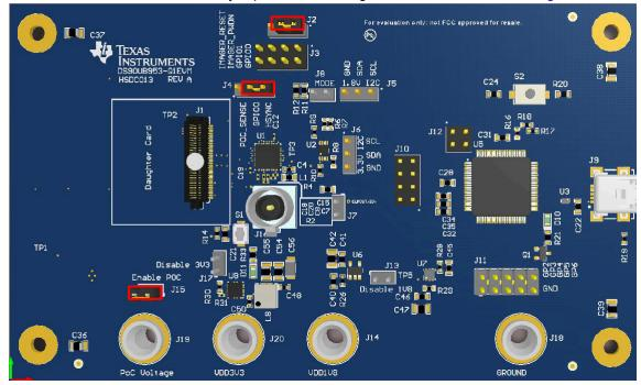
Figure 3-33. DS90UB95x-Q1EVM With Installed Jumpers
