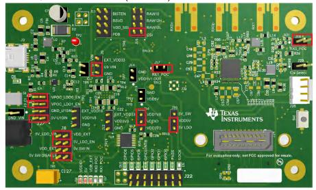
Figure 2-4. DS90UB954-Q1EVM (or variant) With Jumpers Highlighted
