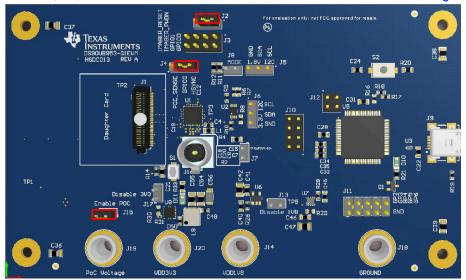
Figure 2-3. DS90UB95x-Q1EVM With Installed Jumpers
