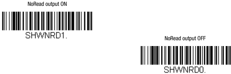
Figure 7.21: Configuration code for switching the NoRead output option on/off
