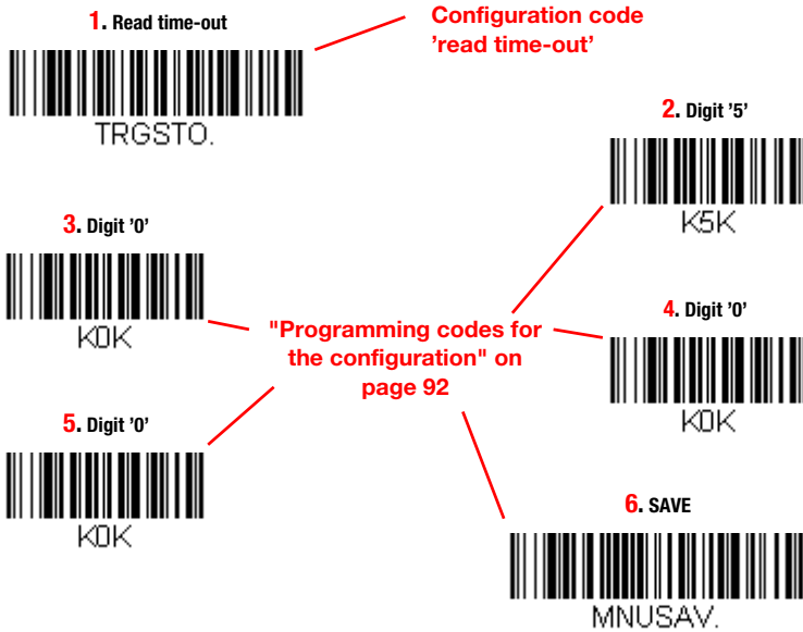
Figure 7.8: Example: Setting a read time-out time of 5 seconds
