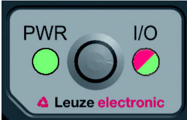
Figure 6.1: LEDs of the LSIS 22x
