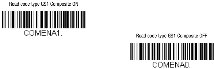
Figure 7.42: Configuration codes for activating/deactivating the GS1 Composite code type
