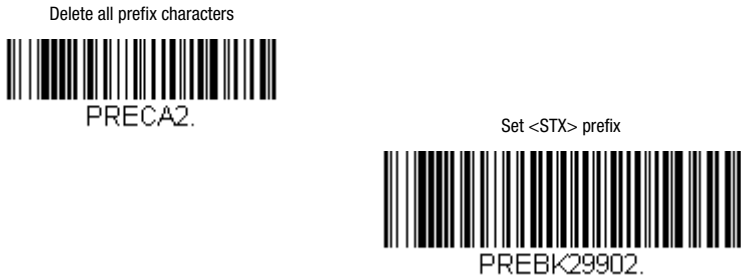
Figure 7.19: Configuration codes for setting the prefix
