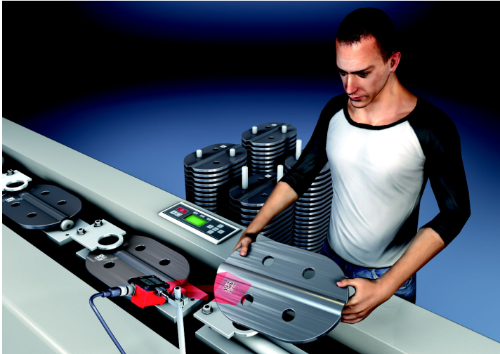
Figure 3.3: Application example: reading 2D-codes in presentation mode
