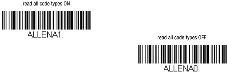
Figure 7.22: Configuration codes for activating/deactivating all code types
