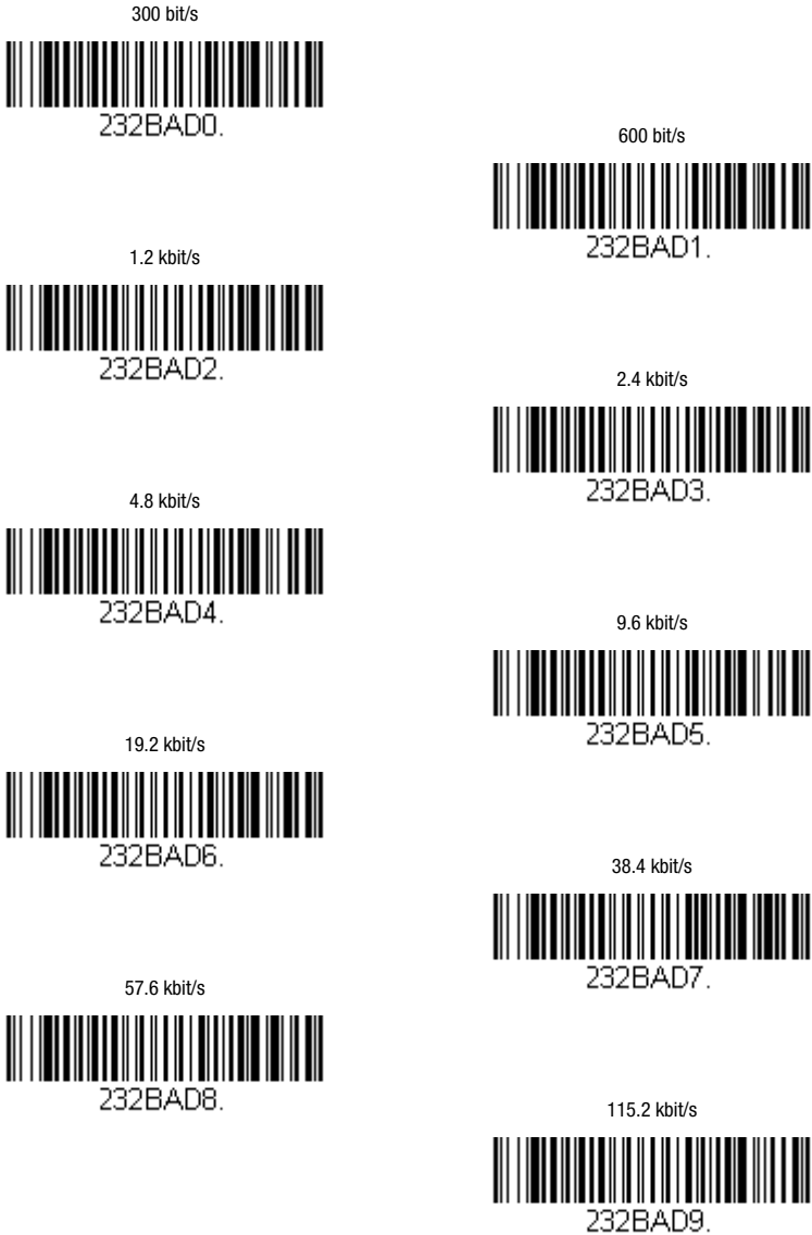
Figure 7.2: Configuration codes RS 232 baud rate
