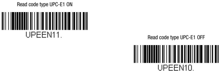
Figure 7.34: Configuration codes for activating/deactivating the UPC-E1 code type
