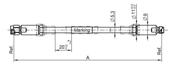
All dimensions are in mm; tolerances:  $\pm$  3mm for A  $\leq$  300 mm;  $\pm$  1% for A > 300 mm\*) If length "A" < 150 mm marking is mount centric  $\pm$ 5 mm
