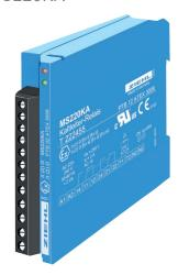
PTC-relay for the application as a protection device against inadmissible heating up at electrical equipment in areas with explosive gases (zones 1 and 2) and areas with combustible dust (21 and 22), e.g. for direct temperature-monitoring of explosion-proof motors EEx e and EEx d.
