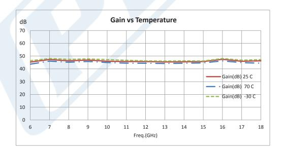
Click the following link (or enter part number in "SEARCH" on website) to obtain additional part information including price, inventory and certifications: 40 dB Gain, 19 dBm Psat, 6 GHz to 18 GHz, Limiting Amplifier, -20 to 20 dBm Pin, SMA PE15A6012
