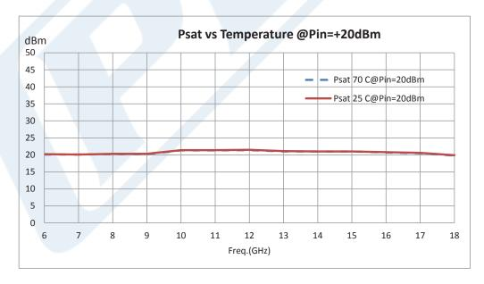
Click the following link (or enter part number in "SEARCH" on website) to obtain additional part information including price, inventory and certifications: 40 dB Gain, 19 dBm Psat, 6 GHz to 18 GHz, Limiting Amplifier, -20 to 20 dBm Pin, SMA PE15A6012
