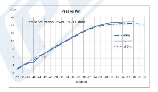
40 dB Gain, 19 dBm Psat, 6 GHz to 18 GHz, Limiting Amplifier, -20 to 20 dBm Pin, SMA from Pasternack Enterprises has same day shipment for domestic and International orders. Our RF, microwave and millimeter wave products maintain a 99.4%
