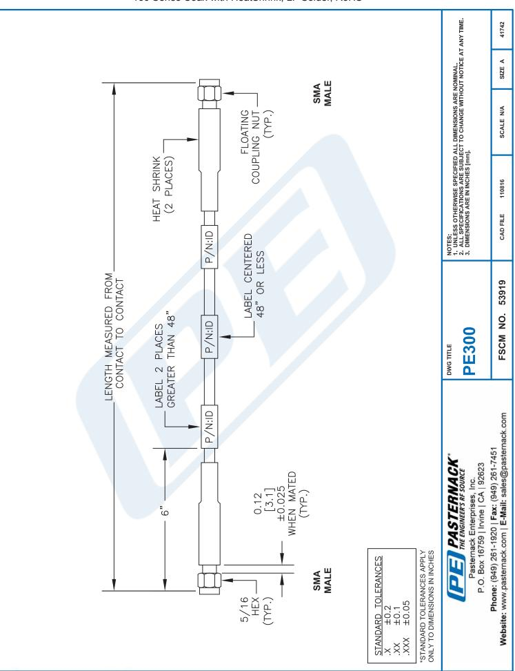
PE300-120 CAD Drawing SMA Male to SMA Male Cable 120 Inch Length Using 160 Series Coax with HeatShrink, LF Solder, RoHS
