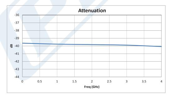
Click the following link (or enter part number in "SEARCH" on website) to obtain additional part information including price, inventory and certifications: 40 dB Fixed Attenuator, N Male to N Female Black Anodized Aluminum Heatsink Body Rated to 25 Watts Up to 4 GHz PE7392-40
