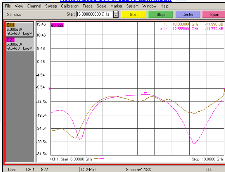
Return Loss S11 & S22 (0 dBm Input)
