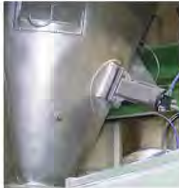
Cleaning bunker walls
