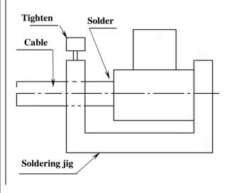
Place cable assembly into a dia D = 3.8 +-0.1 and thickness E = 4 + -0.1.
