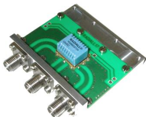
Relay soldered on Test Fixture (2)
