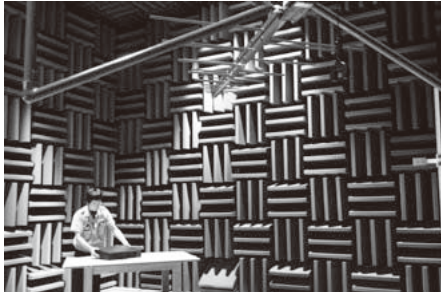
Acoustic radio wave anechoic chamber
