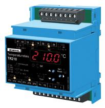
The control unit TR210 monitors up to 2 measuring inputs for Pt100 (RTD), Pt1000, thermocouples, or standard-signals 0/4-20 mA, 0-10 V.
