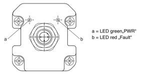
Fig. 7.9-4: Receiver/Transceiver connection cap with LEDs
