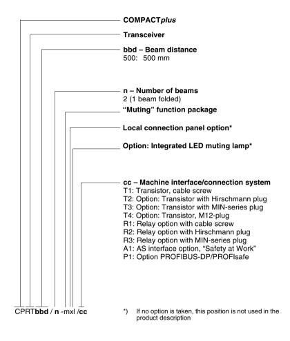
Fig. 1.3-3: Selecting COMPACT plus-m Muting Transceiver
