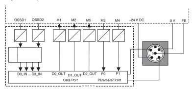
Fig. 7.9-5: Machine interface /A1, schematic structure
