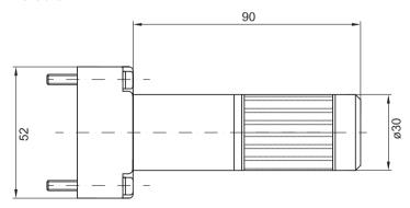
Fig. 12.2-6: Option: Integrated LED muting lamp
