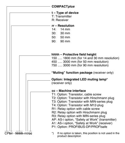
Fig. 1.3-1: Selecting COMPACT plus-m Safety Light Curtains
