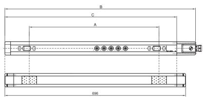
Fig. 12.2-3: Muting transceiver dimensions
