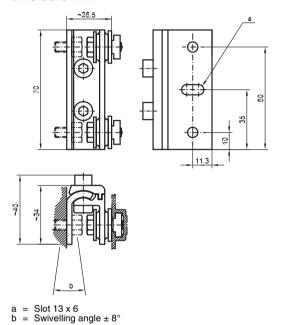
Fig. 12.2-5: Option: Swivelling mounting bracket with shock absorber
