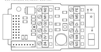
Fig. 7.2-3: Receiver/transceiver machine interface /T1, terminal field
