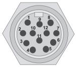
Fig. 7.8-1: Receiver/transceiver machine interface /R3, MIN-series (view of the pins)
