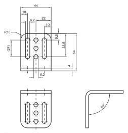
Fig. 12.2-4: Standard mounting bracket
