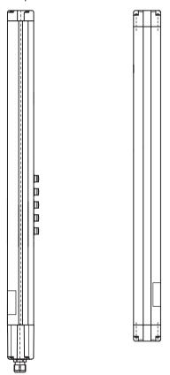
Fig. 9.3-1: Arranging transceiver and passive deflecting mirror
