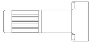
Fig. 3.2-1: Integrated LED muting lamp
